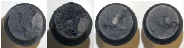
Figure 5. Fracture surfaces of fatigue test (from left to right are 70°C 48h, 70°C 96 h, 120°C 48h, 120°C 96h)
