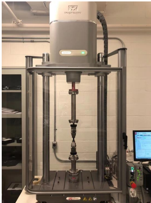
Figure 2. the ElectroPuls E3000 All-Electric Dynamic Test Instrument
