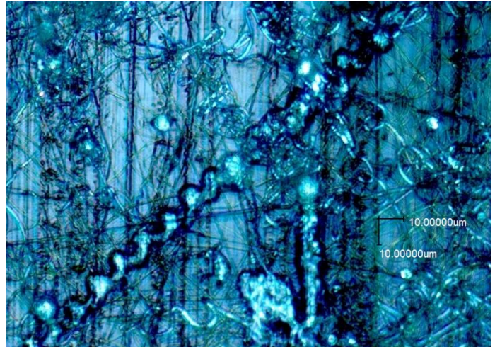
Figure 2 Helix fiber obtained from the following parameters: PCL concentration:15%, TCD:15cm, Flowrate:0.75ml/hr. and collector angle 0^\circ
