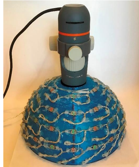
Figure 2. USB microscope above 150 mm diameter 3D printed hemisphere with N = 50 Neopixel strand.
