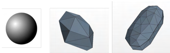
Fig. 6: Particle shapes with aspect ratios from left to right: 1, 1.6 and 2.3
