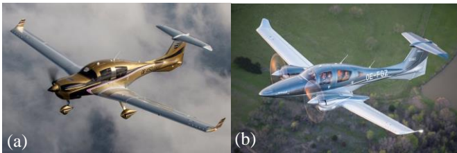
Figure 2. Two different aircraft designed by Diamond company where a. DA-50, is a single engine aircraft b. DA-62, is a twin-engine aircraft designed based on the DA-50 within 6 months [8-9]
