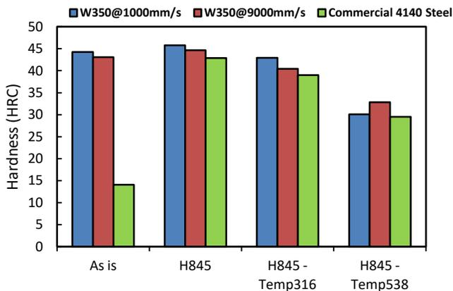
Figure 2. Results of hardness tests (HRC).
