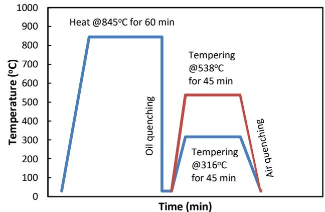
Figure 1. Heat treatment and quenching processes.
