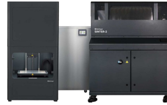
(b) Markforged Metal X System: A new BPE based machine comprised of a printer, wash, and sinter [5].
