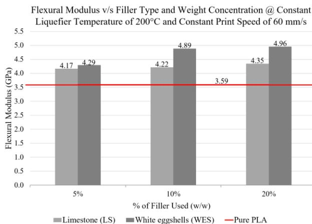
Figure 5. Graph of flexural modulus v/s filler type and concentration % (w/w) for samples printed using a liquefier temperature of 200°C and a printing speed of 60 mm/s.
