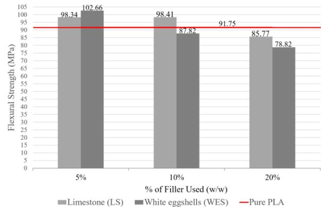
Figure 4. Graph of flexural strength v/s filler type and concentration % (w/w) for samples printed using a liquefier temperature of 200°C and a printing speed of 60 mm/s.
