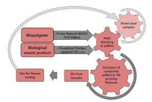
Figure 1. Solid lines: Schematic representation of the process flow for sample preparation and testing in this study. Dotted lines: Insight of next recommended step of closing the material loop by reusing test samples as raw material.
