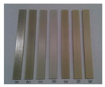
Figure 2. Typical 3D printed flexural specimens (a) pure PLA, (b) 5% (w/w) LS, (c) 10% (w/w) LS, (d) 20% (w/w) LS, (e) 5% (w/w) WES, (f) 10% (w/w) WES and (g) 20% (w/w) WES.
