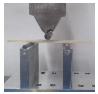
Figure 3. Flexural three-point bending setup following ASTM D790-17 standard used in this study.
