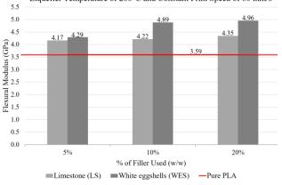
Flexural Modulus v/s Filler Type and Weight Concentration @ Constant Liquefier Temperature of 200°C and Constant Print Speed of 60 mm/s
