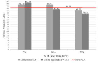
Figure 4. Graph of flexural strength v/s filler type and concentration % (w/w) for samples printed using a liquefier temperature of  $200^{\circ}$ C and a printing speed of 60 mm/s.
