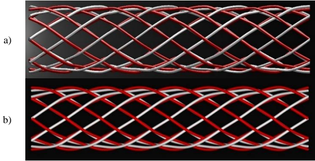
Figure 13 Comparing the result of the generated geometrical TBC model designed by the algorithm developed in this paper a), with the results of the same TBC designed in TexMind Braided software commercial software b). ( N = 16 , \alpha = 35^\circ , R = 10.5 mm, r = 0.5 mm, and the length of the TBC = 98.7 mm)
