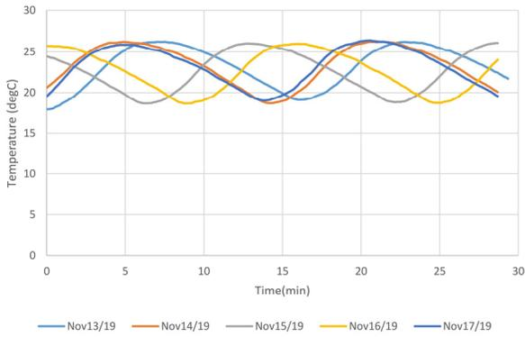
Figure 5. Azimuth actuator temperature throughout flight durations.
