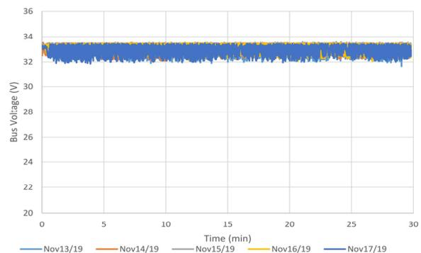
Figure 4. Azimuth actuator bus voltage for demonstration flights.
