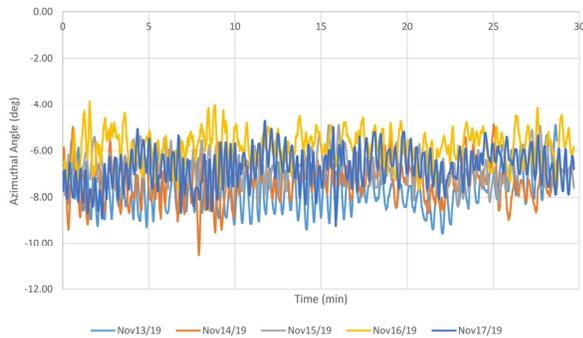
Figure 7. Azimuth actuator range of motion during flights.
