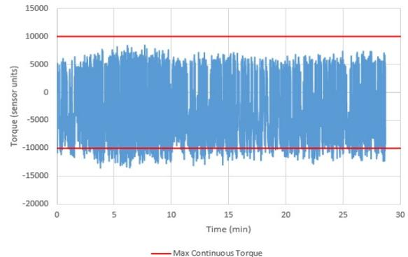
Figure 10. Elevation actuator applied torque during flight.
