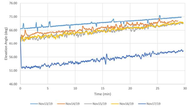
Figure 8. Elevation actuator range of motion during flights.
