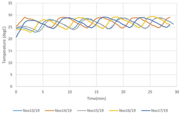
Figure 6. Elevation actuator temperature throughout flight durations.
