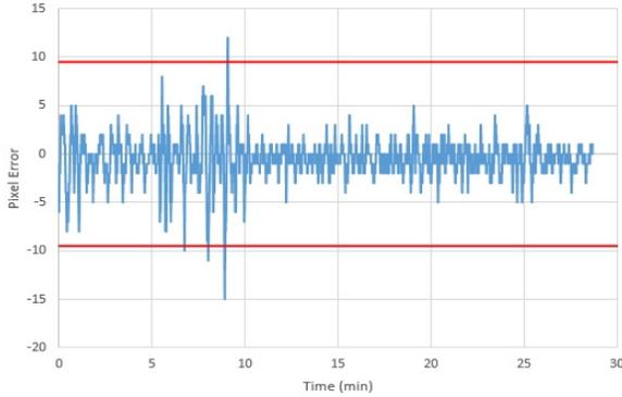
Figure 11. Pixel error in the azimuth axis during flight.
