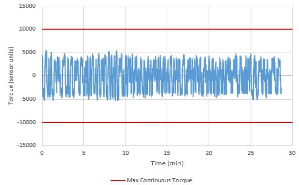
Figure 9. Azimuth actuator applied torque during flight.
