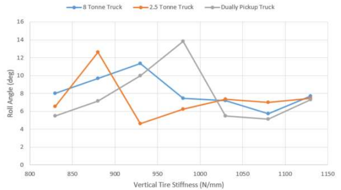
Figure 1. Roll Angle of Trailer at Different Tire Pressures when Driving Straight over 6 in. Half Round
