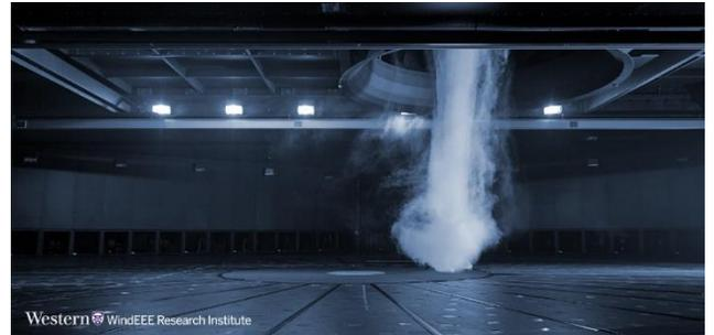
Figure 6: Flow visualization of a tornado in the WindEEE Dome.
