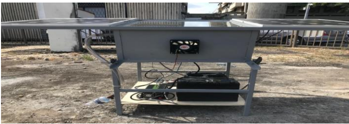
Figure 3: Atmospheric Water Harvesting Device-front view
