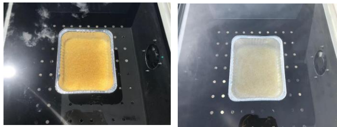
Figure 4: Color change of the indicating silica gel after the Adsorption Process.
