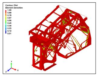
Figure 6: TO results for design refinement (V2), volume fraction = 0.25
