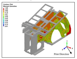
Figure 4: TO results with an overhang constraint, volume fraction = 0.25
