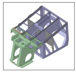
Figure 5: Polymer Pedestal Assembly V1 (C1 = Green, C2 = Purple)
