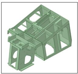
Figure 3: Preliminary Polymer Pedestal Assembly
