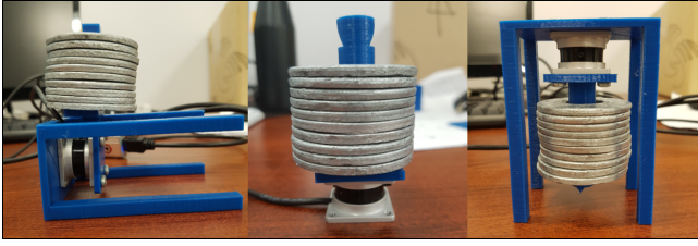
Fig. 2. Test setup for x and y-axes, z-axis in compression, and z-axis in tension
