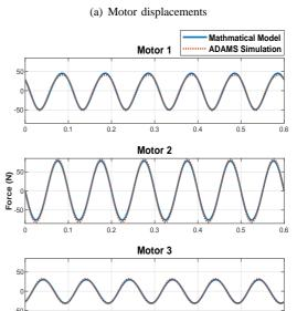
(b) Motor forces Fig. 5. Mathematical model vs. ADAMS simulation under Trajectory 1
