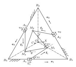
Fig. 1. An arbitrary posture of the 3-PRR planar parallel robot
