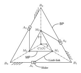
Fig. 2. Reference posture of the 3-PRR planar parallel robot
