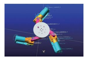
Fig. 4. CAD model of the 3-PRR planar parallel robot in ADAMS simulation
