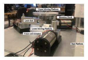
Photo of the prototype of the 3-PRR planar parallel robot
