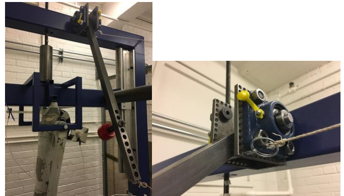
Figure 5. Impact Hammer Assembly (left) and Hammer rested on quick release pin place in one of the holes (right)
