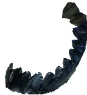
(d) Serrated chip obtained from machining experiments
